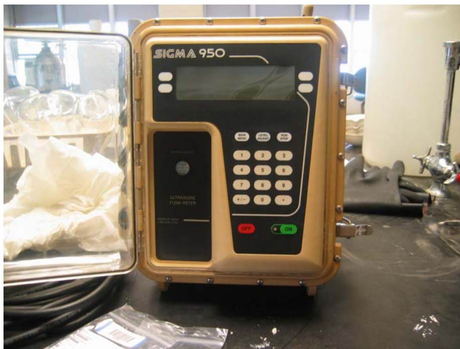
Figure 3.1 American Sigma 950 flow meter.
