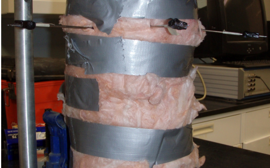
Figure 3.7 Horizontal heat flux: insulated apparatus
