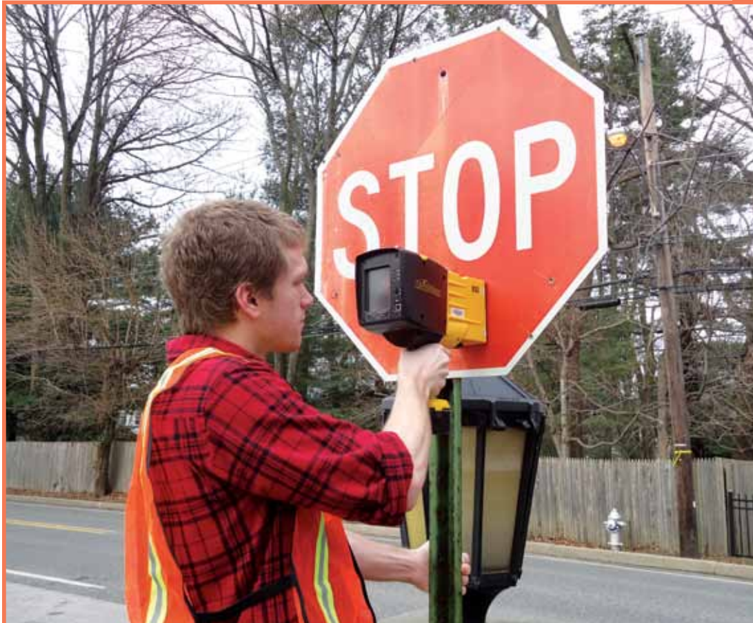
A student is using a retroreflector to conduct field measurements on this STOP sign to support data collection for the sign inventory database. Photo: Vanvi Trieu, Villanova University.
