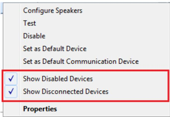
**Step 3)**, Right click the active playback device and select “Set as Default Device.” This will activate the appropriate playback device and allow audio to pass out of your laptop to the AV system. To adjust the playback volume use the instructions in Step 1. Also, please take note of the playback device settings as they may need to be changed again when you connect to a different display or AV system.
