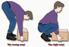
Lift Safely: Bend at the knees lift with the legs
