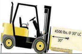
Improperly distributed loads may tip the forklift because the center of gravity has shifted
