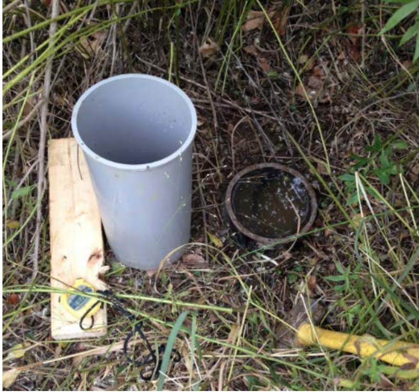
Figure 1.8 A single-ring infiltrometer test
