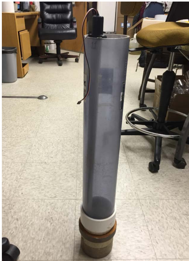
Figure 4.6 A Modified Philip-Dunne infiltrometer with a steel driving ring
