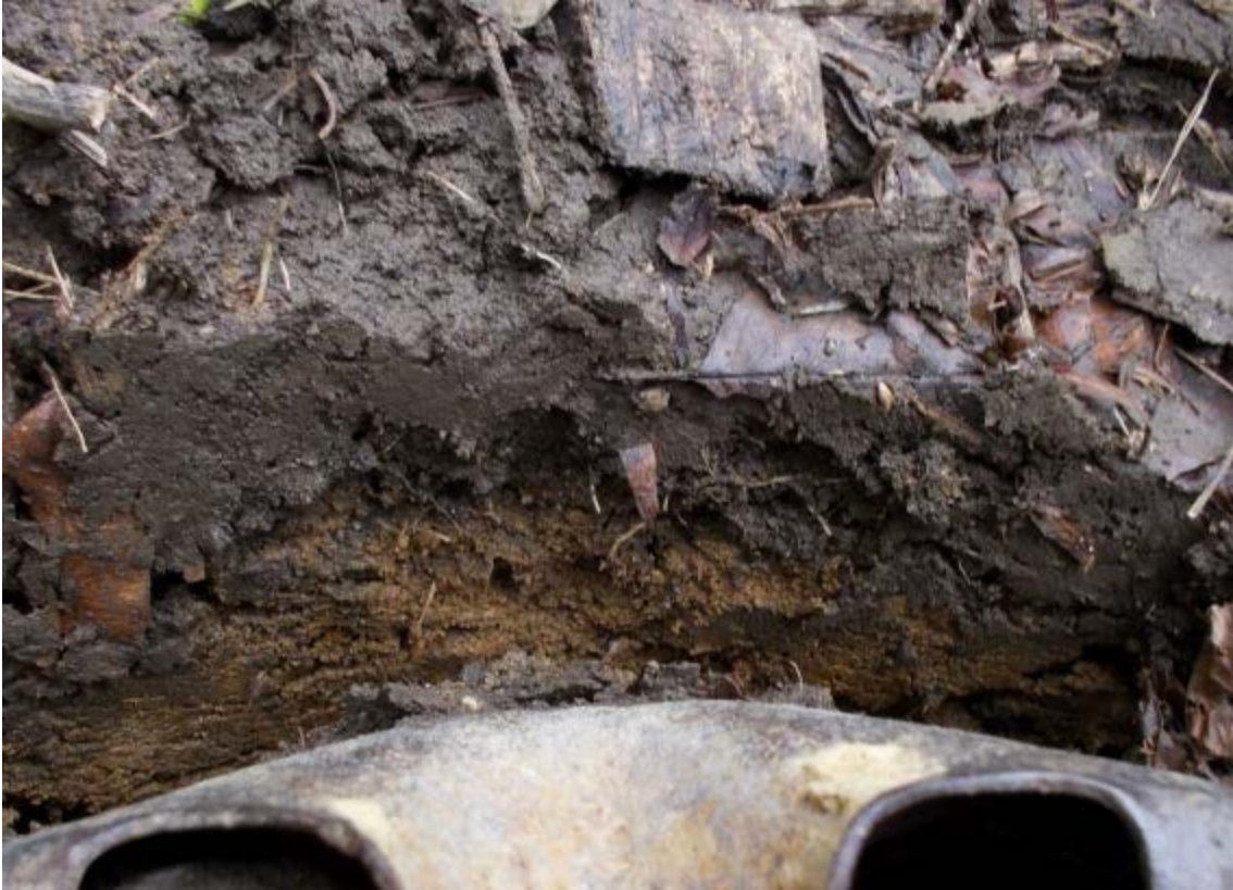
Figure 3.55 The organic layer overlaying the BTI soil mix (Emerson et al. 2015)
