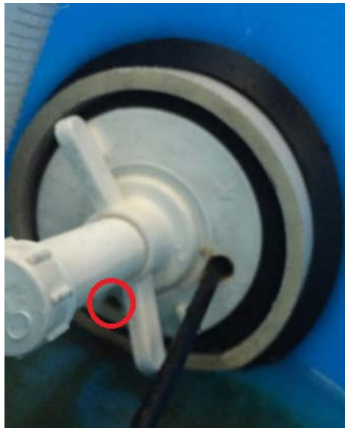
Figure 3.21 The well cap with an orifice installed in the testing apparatus
