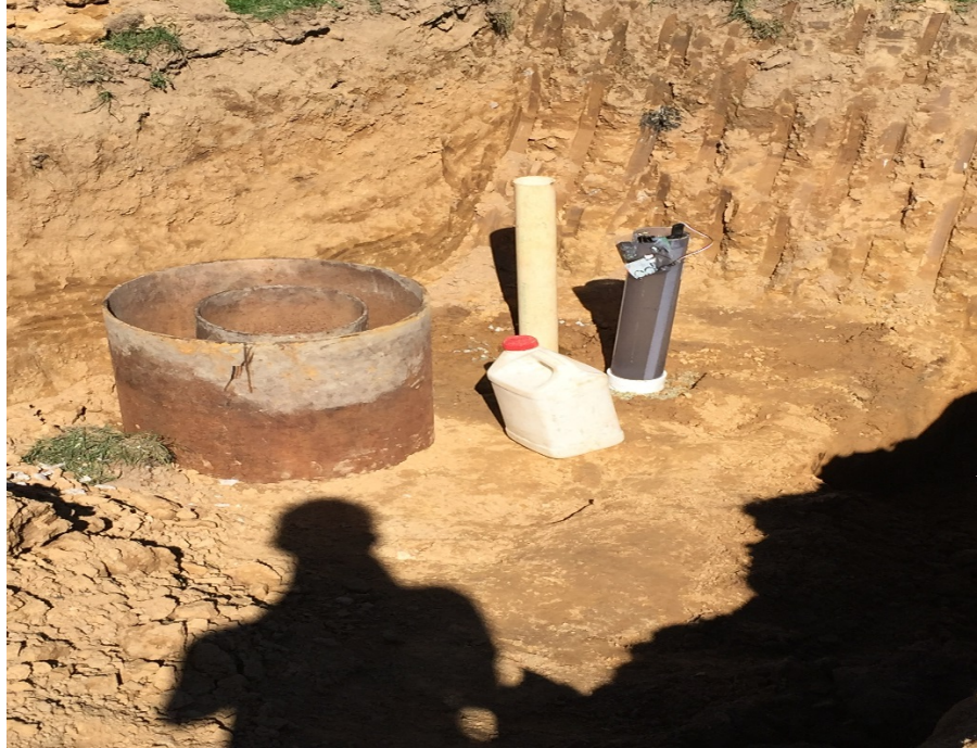
Figure 6.10 Infiltration testing being conducted in a test pit at the Upper Moreland site
