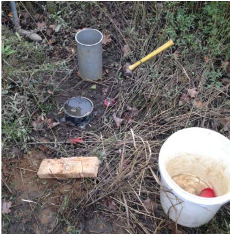
Figure 4.4 A single-ring infiltrometer test with the typical equipment necessary to run the test
