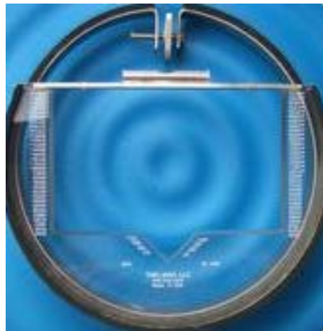
Figure 3.15 An example of a volumetric weir (Thel-mar 2016)
