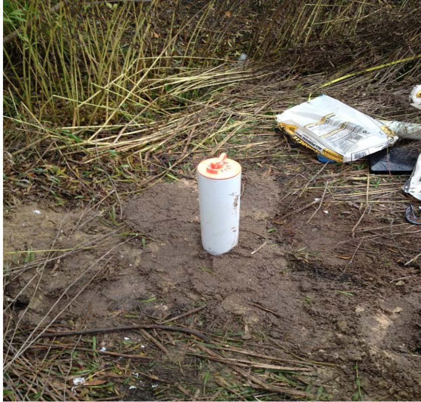
Figure 3.37 The monitoring well in the pond at the PTI
