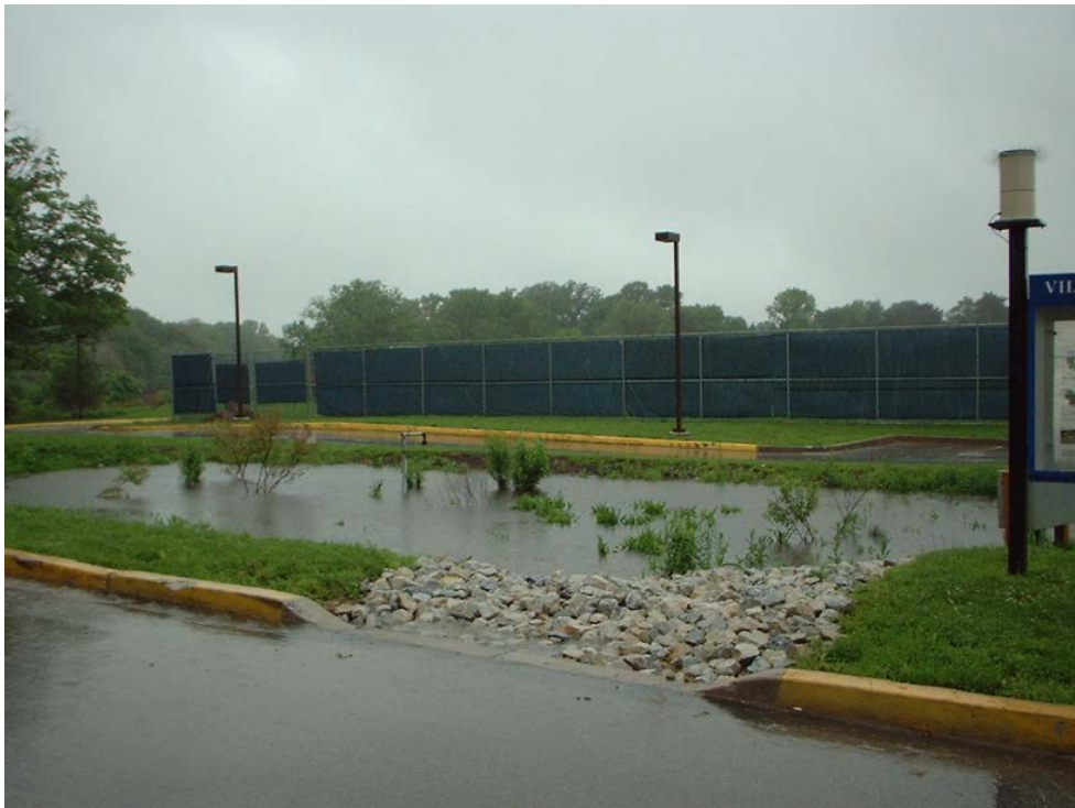
Figure 4.5 A ponding event occurring at the BTI where the recession rate can be determined (photograph courtesy of Villanova Urban Stormwater Partnership)
