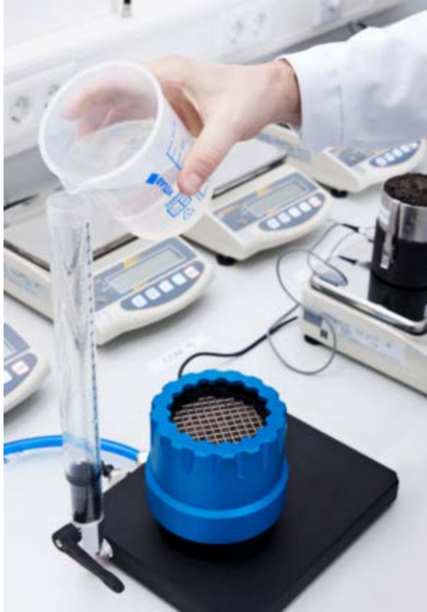
Figure 4.7 A UMS KSAT test (Decagon Devices 2016)
