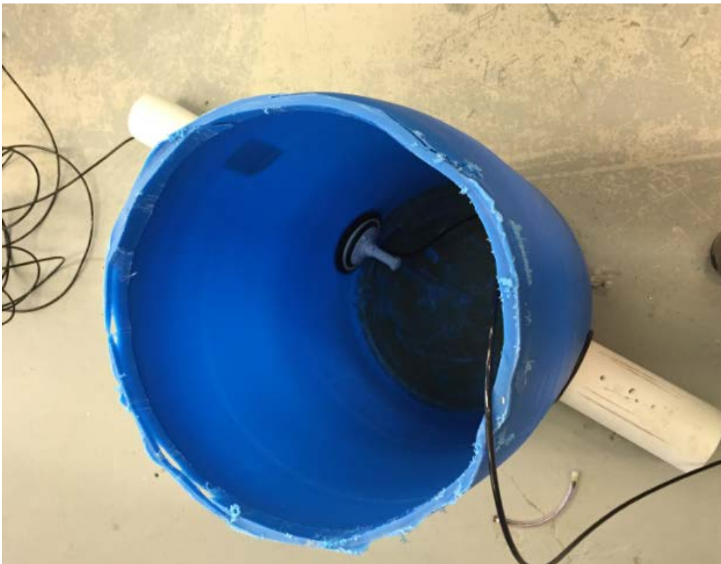
Figure 3.22 The laboratory apparatus used to test the well cap with an orifice
