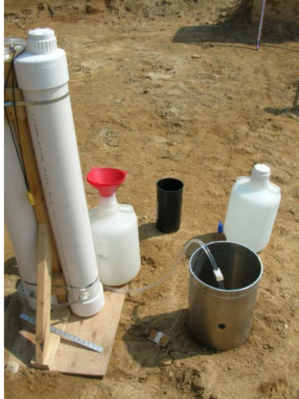
Figure 3.41 Single-ring infiltration test being performed at the PTI (photograph courtesy of Villanova Urban Stormwater Partnership)
