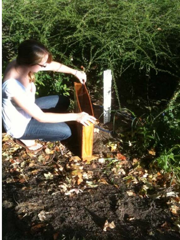
Figure 3.17 Pressure transducer calibration at the FRG (photograph courtesy of Villanova Urban Stormwater Partnership)
