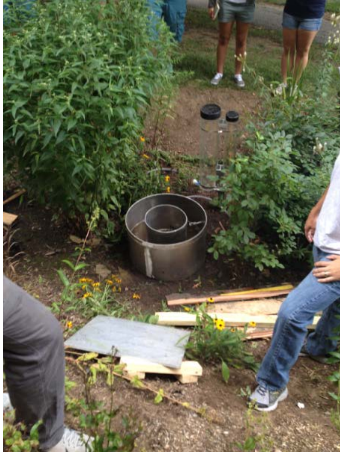
Figure 4.2 A double-ring infiltrometer test being conducted at the FRGI
