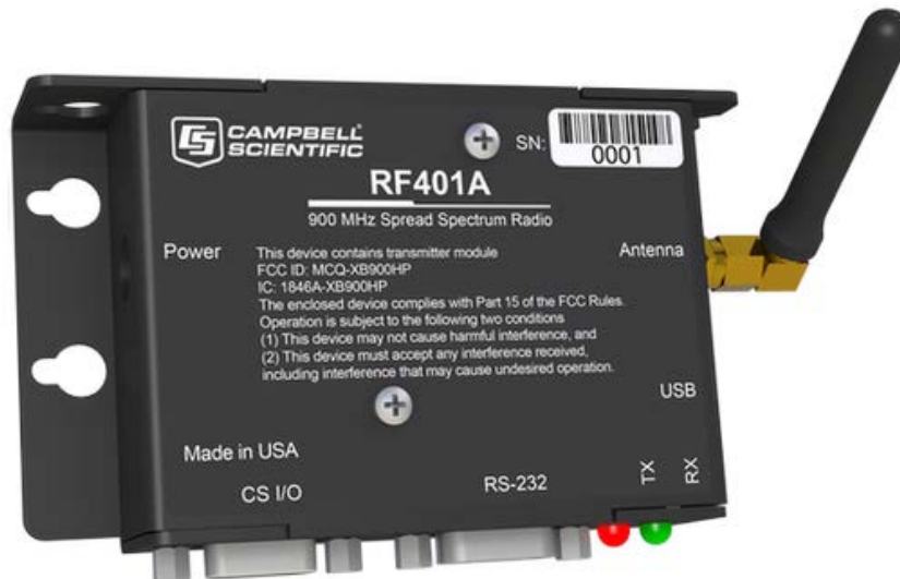
Figure 3.47 Campbell Scientific RF401A spread-spectrum radio (Campbell Scientific 2016)
