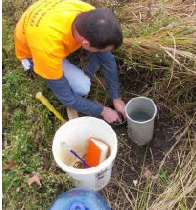
Figure 6.2 A single-ring infiltration test at the BTI (Emerson et al. 2015)
