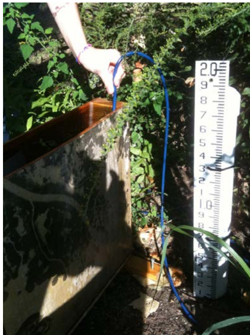
Figure 3.18 A pressure transducer in a calibration container at the FRG (photograph courtesy of Villanova Urban Stormwater Partnership)
