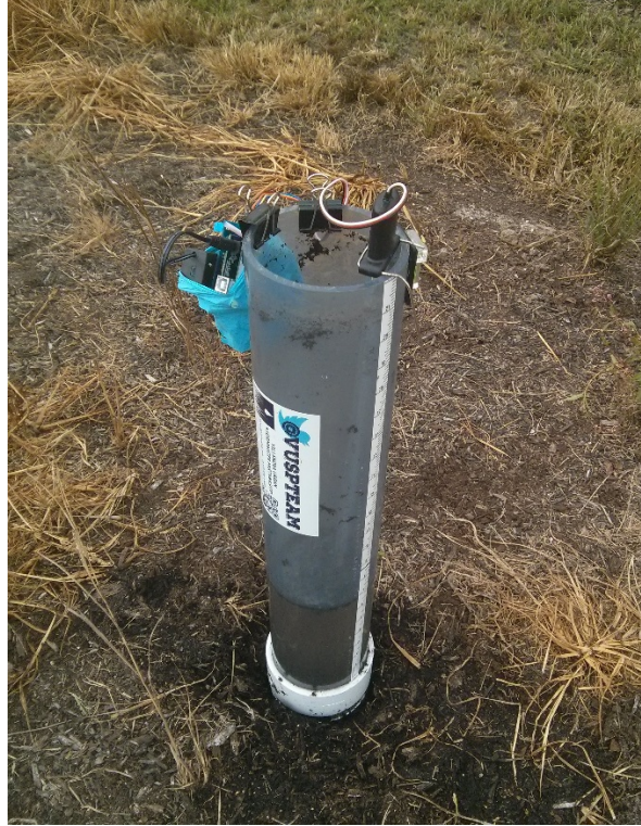
Figure 1.10 The modified Philip-Dunne infiltrometer (photograph courtesy of Villanova Urban Stormwater Partnership)
