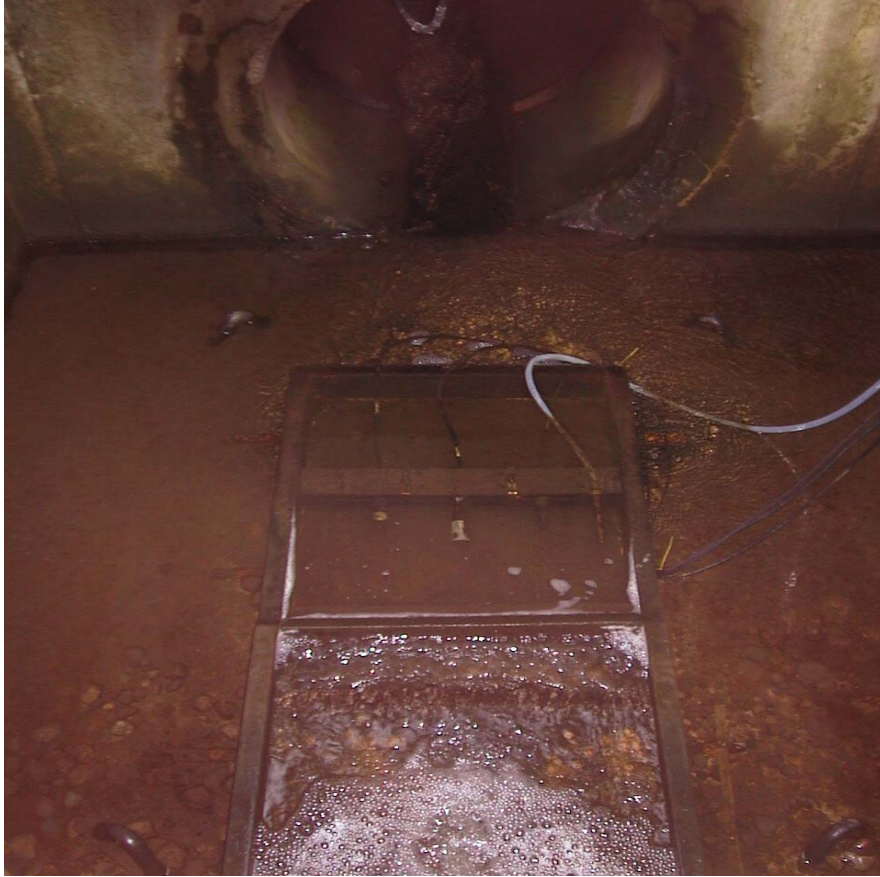
Figure 3.2 Outlet outfitted with pH, conductivity, dissolved oxygen, and sampler.
