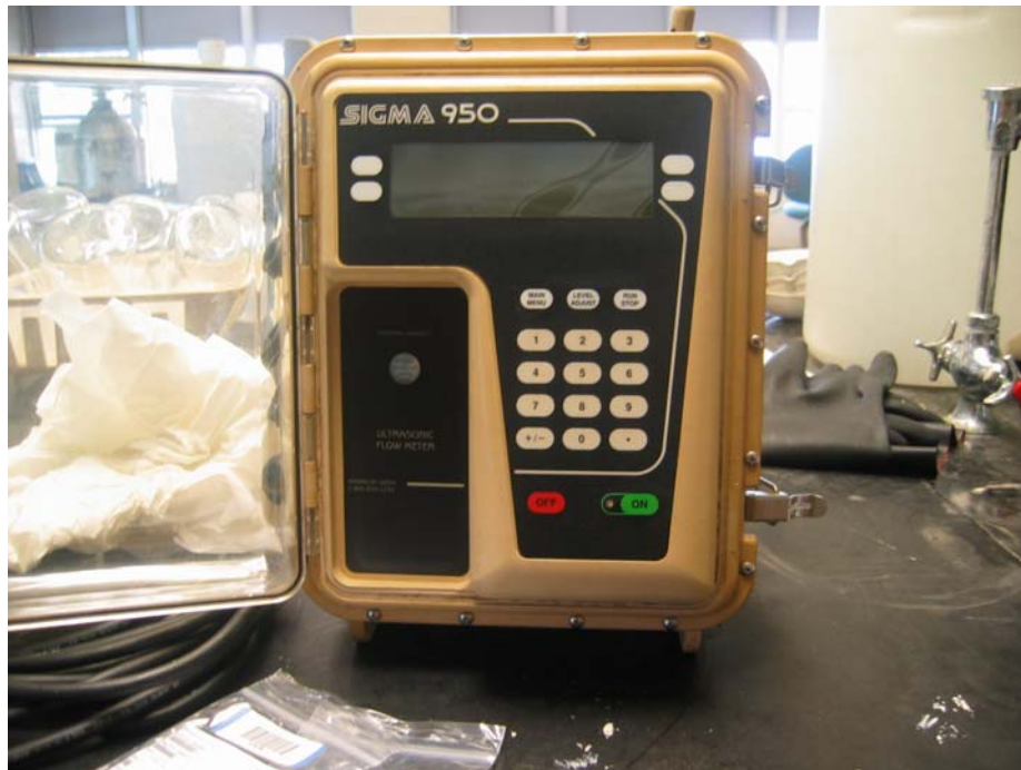
Figure 3.1 American Sigma 950 flow meter.
