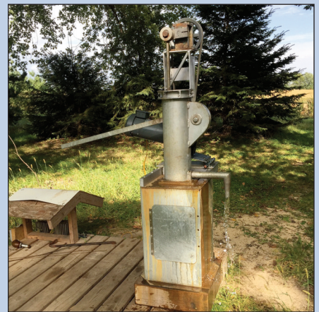
Rittenour's hydraulic hand pump has pumped more than 150,000 gallons of groundwater with more than one million hand strokes without any major breakdown in testing. Photos courtesy Congo Frontline Missions.
