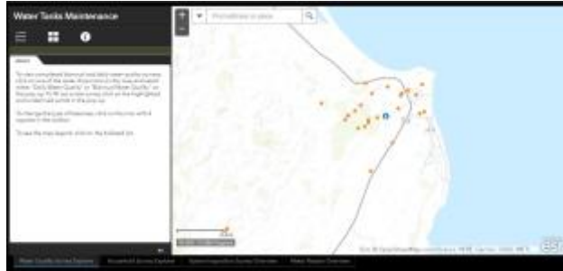
6 - Screenshot of the ArcGIS Dashboard created for CRS. The tab shown here offers water operators and CRS staff the ability to report water quality at various points within the distribution system.
