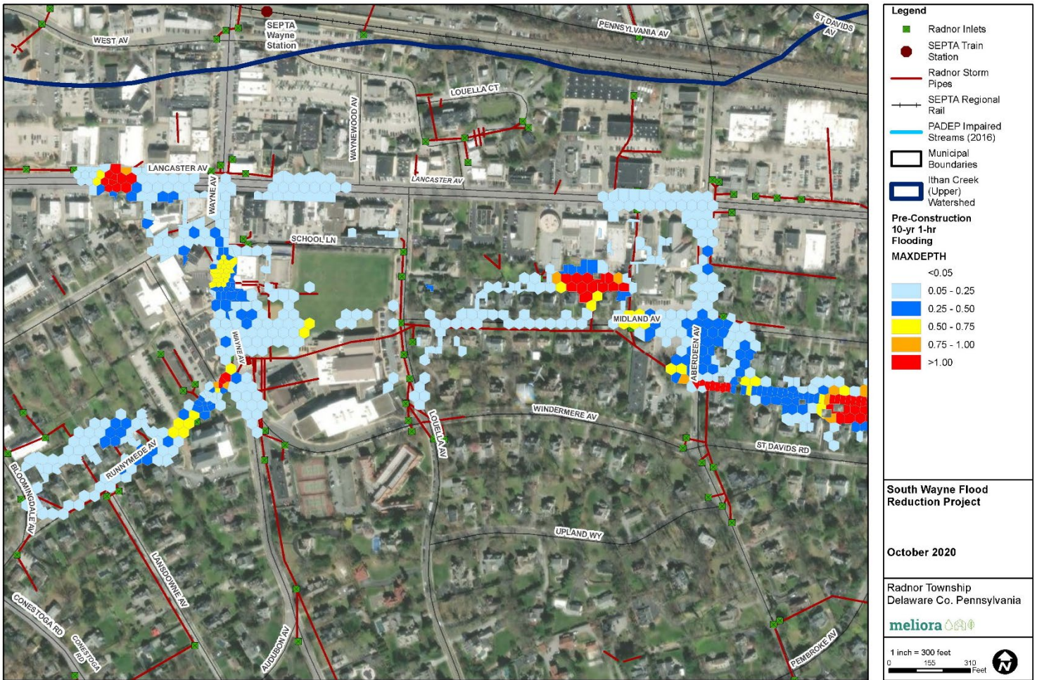
Figure 2 – Modeled max flooding depths during the design 10-yr 1-hr storm in an area of Radnor that has experienced flooding issues
