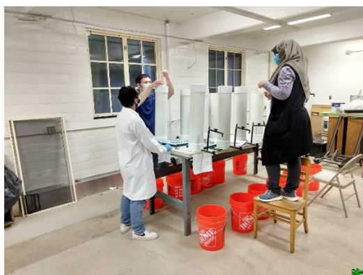
Figure 1. Soil column set-up during measurement of surface greenhouse gas emissions. PVC cap chambers on top of columns facilitate measurement of surface greenhouse gas fluxes over a 30 minute period.
