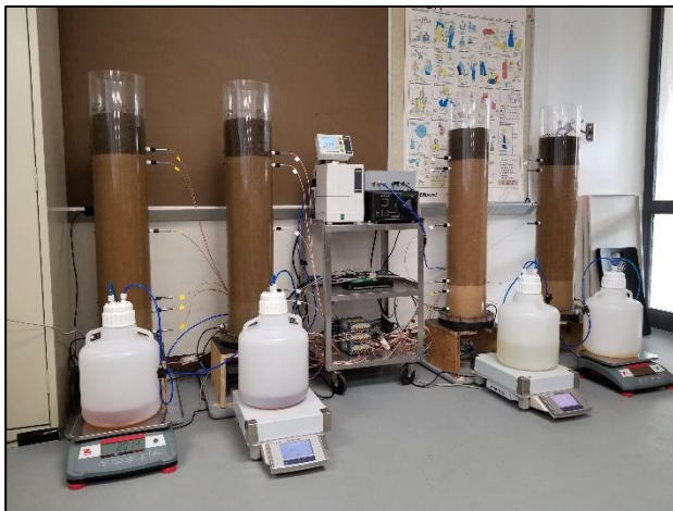
Figure 1. Setup of the mesocosm experiment. Columns vary only in the proportion of glass-sand vs. mined sand within the media.
