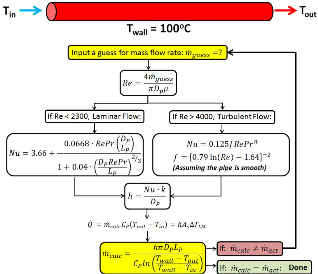
**Figure 3** – Iterative process for determining the mass flow rate required to heat a fluid stream from a specified inlet temperature ( $T_{in}$ ) to a desired outlet temperature ( $T_{out}$ ) using a pipe with a constant wall temperature ( $T_{wall}$ ). Additional variables and properties are inner pipe diameter ( $D_P$ ), length of pipe ( $L_P$ ), Prandtl number ( $Pr$ ), thermal conductivity ( $k$ ), and heat capacity ( $C_P$ ). All equations are adapted from the course textbook.<sup>9</sup>
