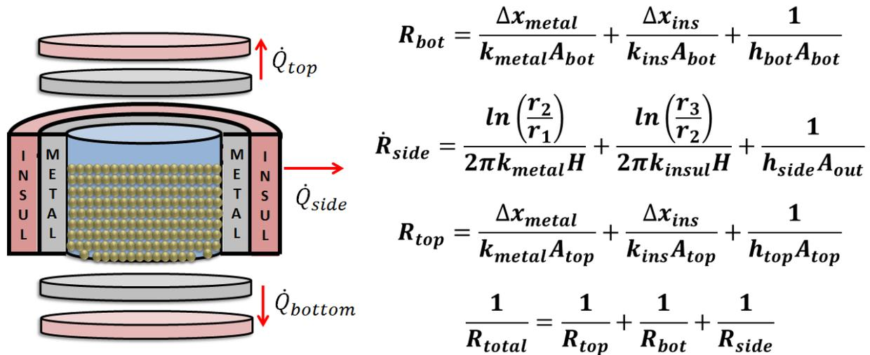
**Figure 4** – Modeling heat loss from an insulated tank (left) can be achieved by estimating the total series and parallel resistances to heat transfer with the equations shown above on the right. Additional variables include surface area ( $A$ ), thermal conductivity ( $k$ ), layer thicknesses ( $\Delta x$ ), inner tank radius ( $r_1$ ), outer tank radius ( $r_2$ ), and outer insulation radius ( $r_3$ ).
