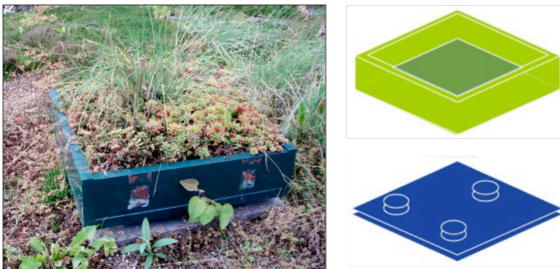
Figure 3.1.3: Picture and schematic of weighing lysimeter used in this research. The lysimeter is 45.7 cm x 45.7 cm x 10.2 cm deep (18"x18"x4"). (Feller 2010)
