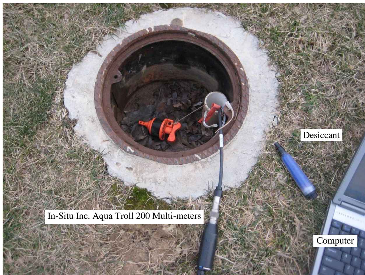
Figure 3.6. Groundwater Well Setup with Aquatroll, Desiccant, and Computer (image courtesy of Villanova University: Villanova Urban Stormwater Partnership)
