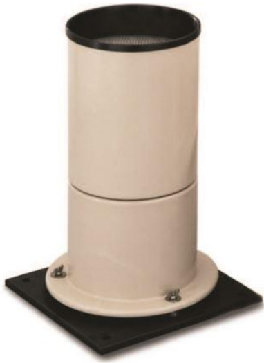
Figure 3.4. American Sigma Tipping Bucket Rain Gauge Model 2149
