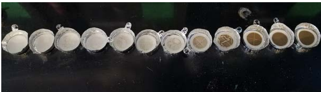
Figure 5-69: TSS Filters after testing (increasing infiltration from left to right)
