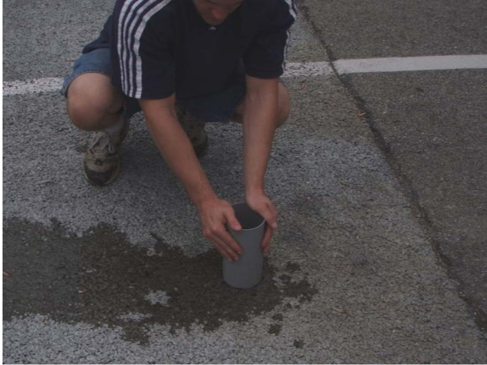
Figure 5-7 Clogged Pervious Concrete
