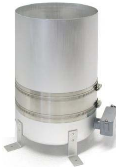
Figure 3-9 Tipping Bucket Rain Gage (Rainwise Inc. 2008)
