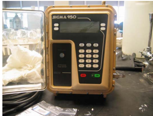
Figure 3.6: Area/Velocity Bubbler with Flow meter
