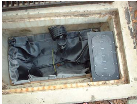
Figure 8.6: Inlet with First Flush and Gutter Sampler
