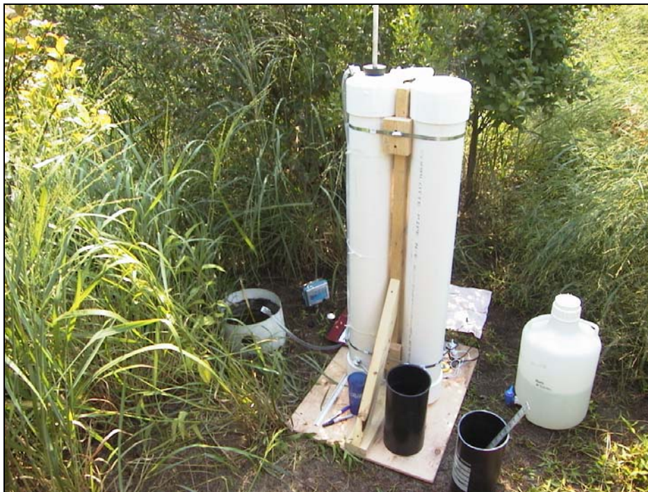
Figure 79. Single-ring infiltrometer experimental setup for the west ring on August 3 rd , 2006.
