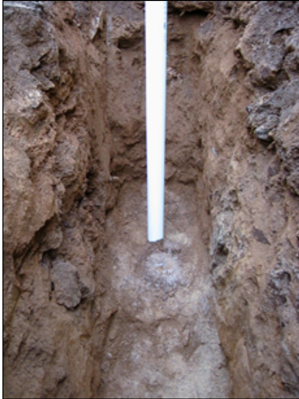
Figure 75. Three inch PVC pipe installed for Maryland infiltration test.
