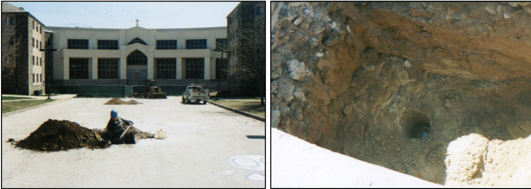
Figure 69. Location of two test pits (left) and an ongoing infiltration test in one of the test pits (right).
