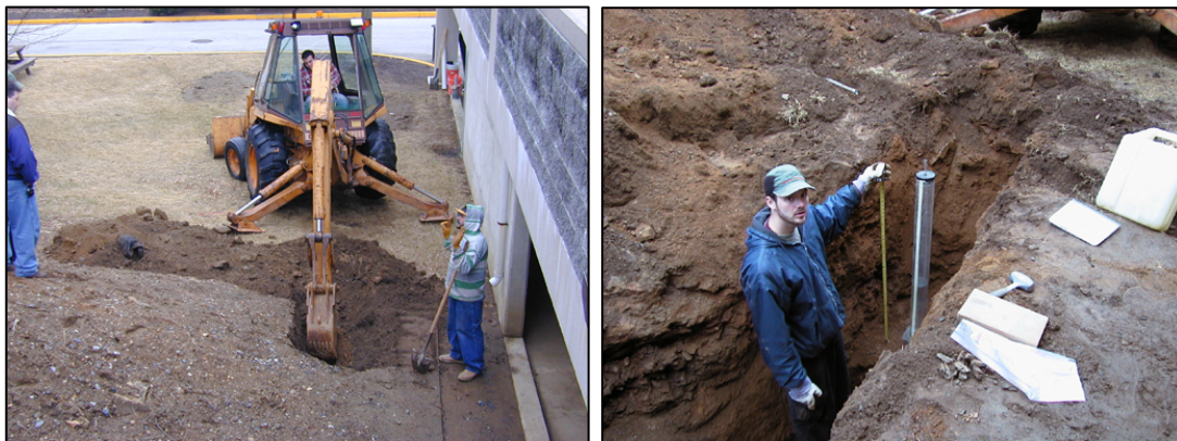
Figure 73. Test pit location and fully excavated pit during constant head infiltrometer test.
