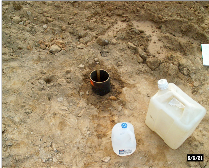
Figure 71. Ongoing infiltration test at the BTI.
