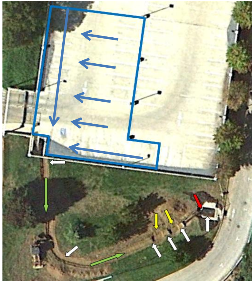
Figure 1.1 - Aerial of the treatment train (Adapted from Google Earth) Green, yellow, and red arrows signify the swale, rain gardens, and infiltration trench, respectively. White arrows indicate monitoring and sampling points.
