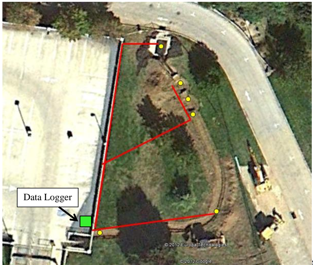
Figure 4.6 - Diagram of pressure transducer and sensor conduit to data logger (Yellow dots represent pressure transducer locations and red lines indicate their wiring route)
