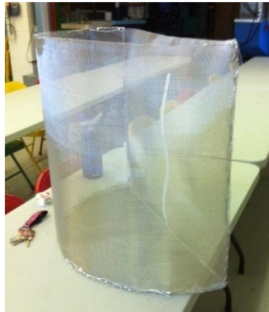
Figure 3.14 - Basket to catch debris prior to infiltration trench
