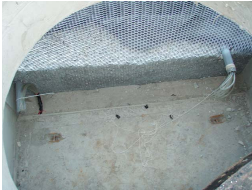
Figure 3.2: Access box with screen facing infiltration bed, and tubing from pore water samplers.
