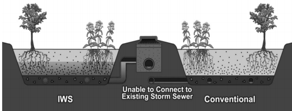
Figure 2.2: Internal Water Storage vs. Conventional Drainage (Brown et al. 2009)
